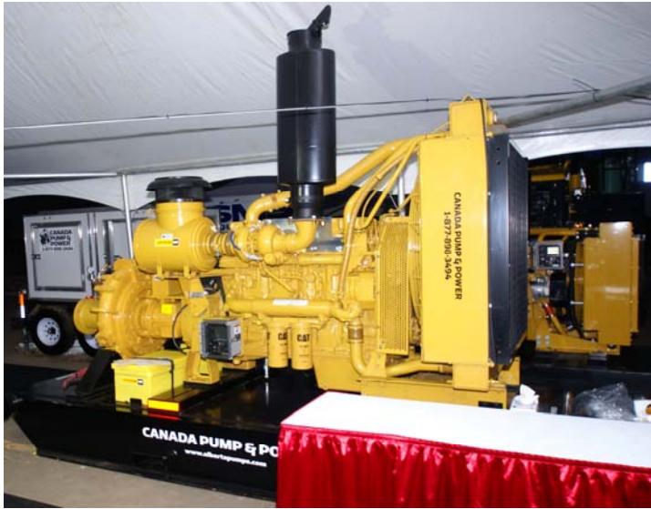
8" High Head Water Pump – 600 HP
