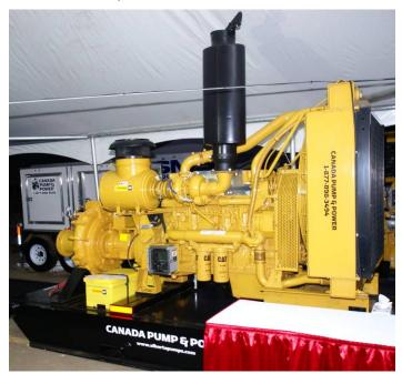
Each HW8 is capable of a max head of 660 feet (200 meters) and max flow of 3,970 gpm. Built with a Cornell 6822MX pump end and a CAT C18 high efficiency diesel engine, they burn less fuel than most pumps. Installed with a LOFA panel and messenger unit, the pumps can be remotely monitored and controlled by any computer with internet access.
