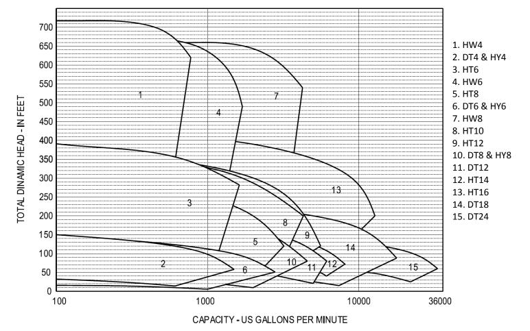
\*Size pump to center of the curve. Operating on the edges of the curve is less efficient.
