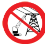
Do not work under or near overhead electric power lines
