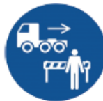
Position yourself in a safe zone in relation to moving equipment
