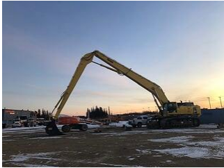
Long Reach Excavators
