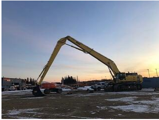
Long Reach Excavators
