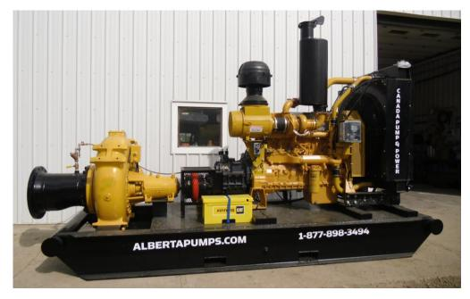
In June Canada Pump and Power received a call from the Suncor Oil Sands with an urgent request to install two of our 18" DT18 Dewatering Trash Pumps at their Low Lift Pump House. Their existing pumps flooded due to high water. CPP performed an emergency installation over the weekend to keep the plant from shutting down.
